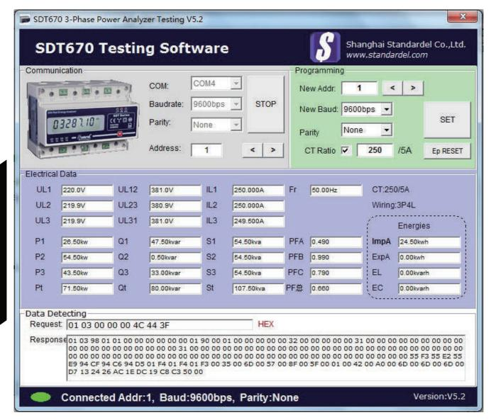
SDT670 Testing Software can check all the state of SDT670 by RS485 communication:
