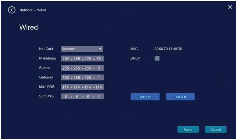
Attention: If not familiar about the LAN environment or the device is in private network, user can turn on "DHCP", which ensure gaining IP address automatically. If familiar about LAN, user can set it and DNS manually to connect to internet.
