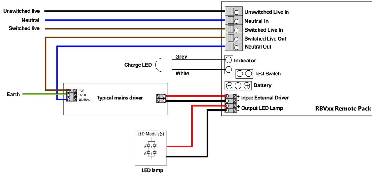
External wiring connections (With jack connectors)
