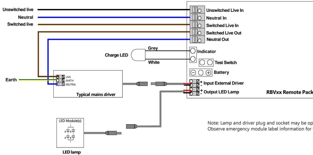
Note: Lamp and driver plug and socket may be opposite gender or different type. Observe emergency module label information for wiring!
