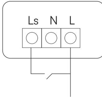
For Maintained Operation - Maintained operation, link L (Switched Live) to terminal Ls (permanent Live). If 'Ls' is not connected, the fitting works as non-maintained
